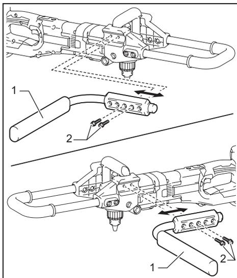
► 1. Bar of the reaction receiver 2. Bolt C
