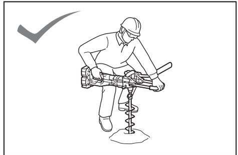
**⚠ CAUTION: Hold the tool firmly.** The tool may back out abruptly and cause an injury.
