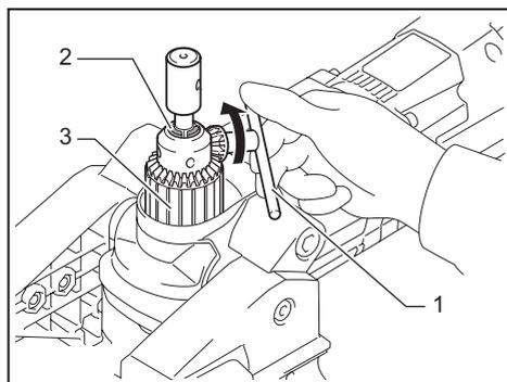
After use, return the chuck key to the storage cavity on the tool as illustrated.
