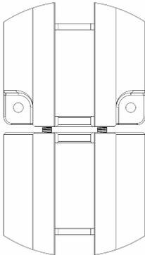
Do NOT fully tighten the cap screws at this stage, but tighten enough so that the add on bed extension is secured to the end of the lathe.
