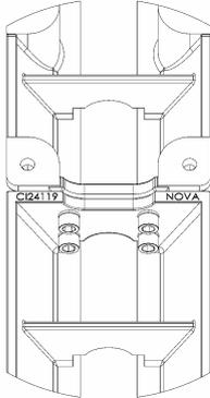
5. Check that the tailstock runs smoothly over the mating joint, and also over the full length of the extension. Although all components manufactured by Teknatool International are made to closest possible tolerances, it is possible for a difference of approximately 0.1mm to put the bed 'out of true'. The tailstock can bind in any given area in two possible ways:
