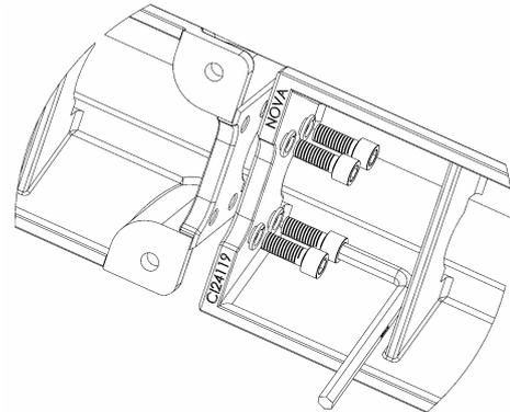
3. Move the tailstock over the two joining extension beds (tailstock approximately covering equal length on either extension). Lock the tailstock firmly over the joining faces.
