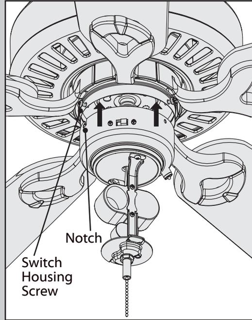
Align the notches in the sides of the lower switch housing with the upper switch housing screws. Lift the lower switch housing. Twist the lower switch housing clockwise to lock into place. Then thread the fan pull chain through the hole in the light kit.
