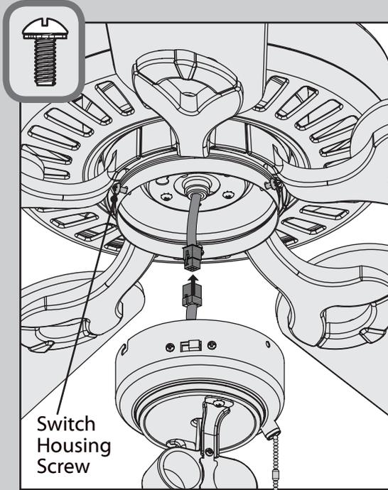
Partially install two of the switch housing screws found in the
