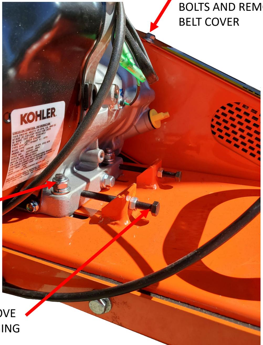
LOOSEN 4 ENGINE MOUNTING BOLTS
