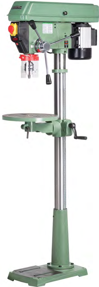
#75-155 | 15" variable speed drill press
