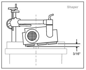
Figure 17 (Stock Feeder in edgewise position)
