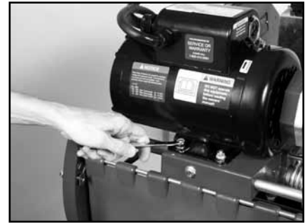
(C) Clean the remainder of the MK- 2000. Verify all Motor Mounting Bolts are tight.
