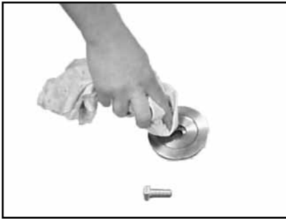
(A) Clean the Outer Flange and Retaining Screw.
