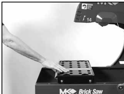
(B) Verify the Movable Cutting Table moves freely along the guide rails.
