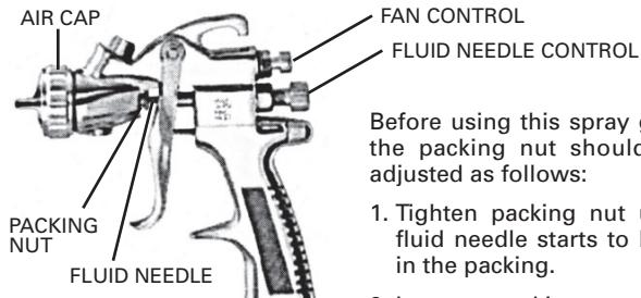
Before using this spray gun, the packing nut should be adjusted as follows:
